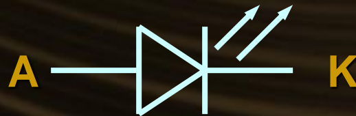
Schematic Symbol for a Light-Emitting Diode
