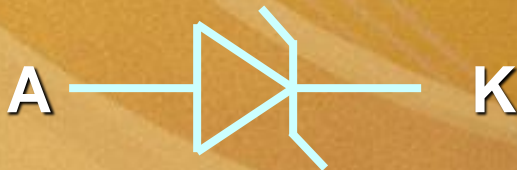
Schematic Symbol for a Zener Diode
